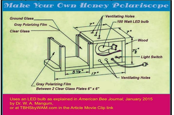
When you install the polarizing filters, make sure they are crossed, so no light comes through them. That blackness removes the background glare. See my January 2015 ABJ article for more details on getting the filters. Note: these are special polarizing filters, not just gray pieces of plastic.
