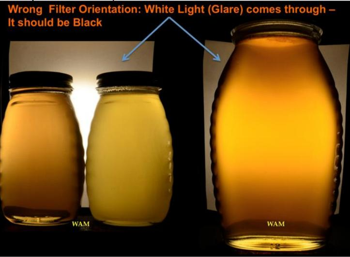
A "regular" one-bulb polariscope is fine for viewing honey, but my camera has different light sensitivities making a bright band in the middle of the jar.
