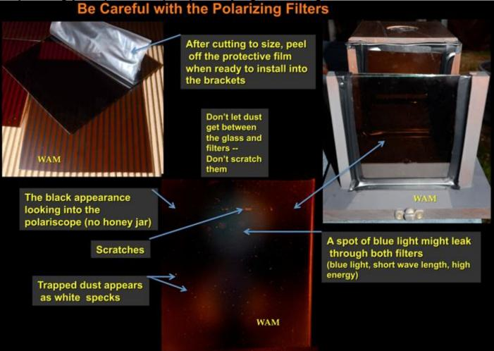
If the polarizing filters are not crossed, white background light (glare) comes through (because the filters are in a parallel orientation).
