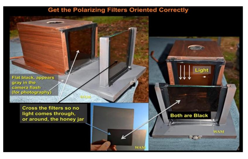
The polarizing filters come covered in a cloudy plastic protective film. Peel the film away right before installation. As shown in the plans above, glass covers the filters on both sides. Any trapped dust or scratch on the filters might appear as white marks. Usually it is not much of a problem, unless like me, you keep taking your polariscope apart, trying new things with it.
