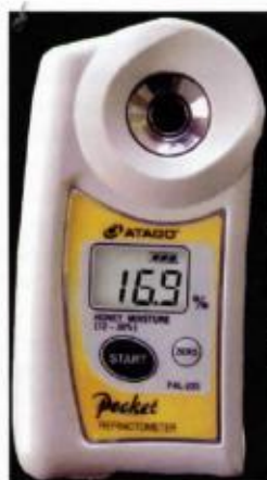
Hand held, and now digital refractometers are available.
